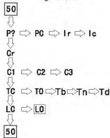
When the actuator has been installed on the valve, limit must be set prior to electrical operation. Limit setting is one of the most important commissioning works. The purpose of it is to store the set data of valve travel range into memorizer.
