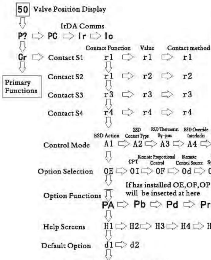
To access the Secondary menu, press "Downward" to find Procedure Branch Crossroad[Cr], then press "Rightward" to find [r1] according to the instruction of picture 4.5.1.
